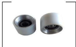
HDRL015 Handrail Support Roller OD70mm W50mm 6204
