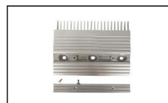
KOAC010 ID:DEE1718890 Comb AL L201.5mm W173mm Hole Space 153mm LHS 22T
