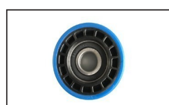
SCRL024 ID:SMS405029 Step Chain Roller OD76mm W25mm 6204-2RS
