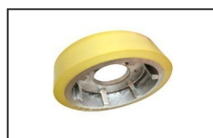
MIRL006 ID:YS011C272G01 Drive Roller OD132mm W35mm ID45mm
