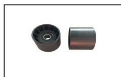
LSRL007 Handrail Support Roller OD70mm W60mm 6202
