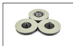
MILR001 Door Hanger Roller OD72mm W15mm 6202
