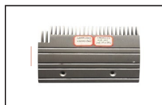
OTAC002 ID:GAA453BM3 Comb AL L206.4mm W139.2mm Hole Space 101.7mm LHS 24T
