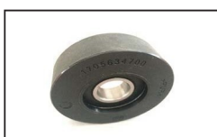
KORL002 ID:DEE3685362 Step Chain Roller OD75mm W23.5mm 6204-2RS
