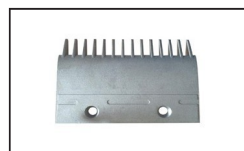
MIAC003 ID:YS017B313 Comb AL L126mm W94mm Hole Space 64mm 14T
