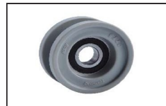
OTRL017 ID:DAA456AG2 Handrail Guide Roller OD70mm W34mm 6203
