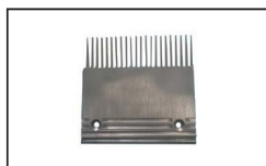
TOAC002-2 Comb AL L199mm W181mm Hole Space 145mm CTR 22T
