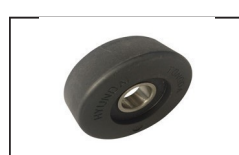
HDRL002 ID:C6500068 Step Chain Roller OD76mm W25mm 6204-2RS
