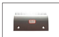
OTAC013 ID:HA453S3 Comb AL L202.9mm W133mm Hole Space 145mm RHS 22T
