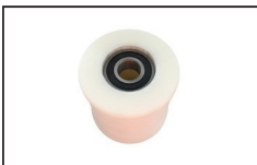
SCRL010 ID:SMH244011 Belt Roller OD89mm W70mm 6204-2RS
