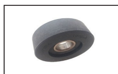
LSRL001 ID:DSA3003675 Step Chain Roller OD70mm W25mm 6204-2RS
