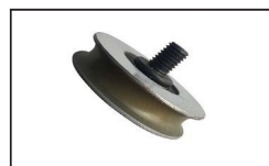
TKLR003 Door Roller OD56mm W14mm 6201RS W L16mm Shaft
