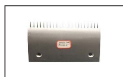
OTAC011 ID:HA453S1 Comb AL L199.4mm W133mm Hole Space 145mm CTR 22T
