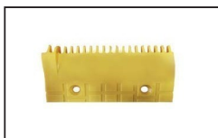
HTPC001 ID:H2200122 Comb Plastic L163mm W90mm Hole Space 90mm LHS 19T
