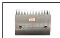
SCAC003 ID:50641440 Comb AL L205.4mm W180.8mm Hole Space 145mm LHS 22T
