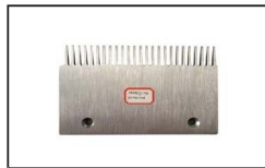
OTAC025 ID:XAA453J3 Comb AL L214.2mm W145mm Hole Space 142.8mm LHS 25T
