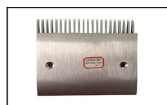
SCAC013 ID:SLR266475 Comb AL L199.4mm W181.36mm Hole Space 145mm RHS/CTR 22T
