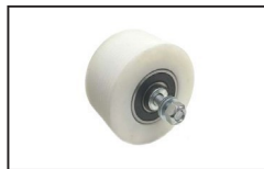
TKRL016 ID:1709154200 Belt Roller OD110mm W60mm 6305-2RS
