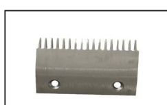
LSAC010 ID:DSA2001559-M Comb AL L142.8mm W91.6mm Hole Space 90mm CTR 17T
