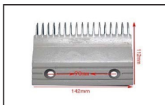
HTAC003 ID:22501789A Comb AL L142mm W112mm Hole Space 90mm CTR 17T
