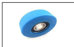
TKRL002 ID:1705060100 Step Chain Roller OD75mm W23.5mm 6204RS
