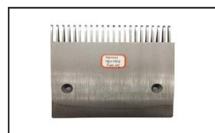
SCAC004 ID:50641441 Comb AL L199.4mm W180.8mm Hole Space 145mm RHS/CTR 22T
