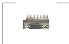
HDAC009 ID:655B013H15,LHS 15T Comb AL L153mm W86.5mm Hole Space 92mm LHS 15T
