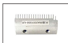
LSAC009 ID:DSA2001558-L/R Comb AL L147mm W91.6mm Hole Space 90mm RHS 17T
