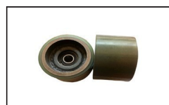
HTRL003-1 Handrail Support Roller OD90mm W60mm 6202
