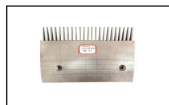
FJAC002 ID:FPA0105 Comb AL L214.6mm W154.3mm Hole Space 145mm LHS 23T
