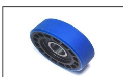
KORL004-1 ID:DEE4008754 Step Chain Roller OD75mm W23.5mm 6204RS
