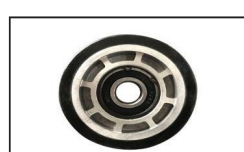
KORL021 Step Roller OD100mm W25mm 6204-2RS
