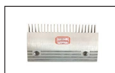
KOAC005 ID: 5130668D10 KM5130668H01 Comb AL L202.2mm W127.2mm Hole Space 140mm RHS 22T
