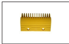
MIPC003 ID:YS017B313 Comb Plastic L127mm W93mm Hole Space 64mm 14T yellow
