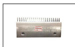
SCAC010 ID:57410421 Comb AL L202.9mm W107mm Hole Space 145mm RHS 22T
