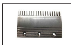
TKAC006 Comb AL L204mm W115mm Hole Space 67mm 24T
