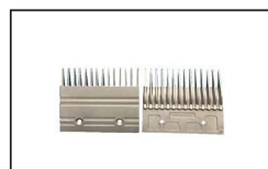
MIAC001 ID:C751001B202 Comb AL L127mm W123mm Hole Space 64mm 14T
