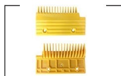
HDPC002 ID:655B013H06 ABS Comb L153mm W86.5mm Hole Space 92mm RHS 15T
